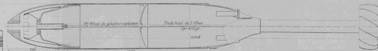
Fig. 9. Projectile de 3<sup>m</sup>353 de longueur.
