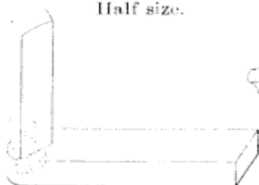
FIG. 28.— Folding-wedge Gauges for Measuring Type-moulds (taper 1 in 100). Full size.
