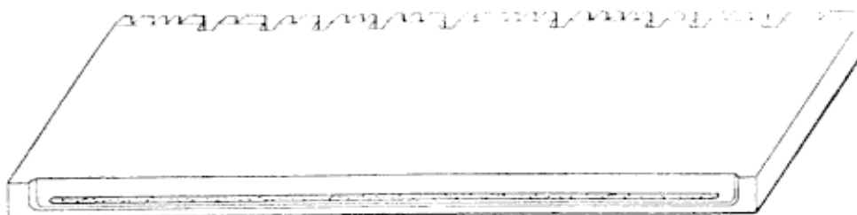
FIG. 116.— Type-slug finished. Full size.
