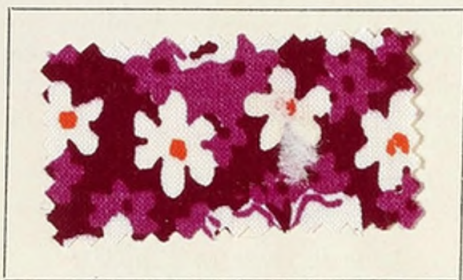
15 gr. Naphtol AS 40 gr. Sel d'Orange solide RDA 40 gr. Sel de Bordeaux solide BD, coupure 1:4
