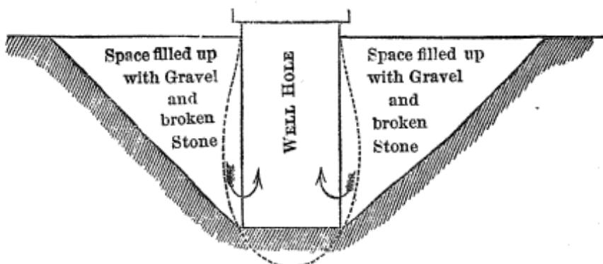
A conical hole is cut out of the ground to a sufficient depth and then a cylinder of brick or stone is built as a well hole, appertures being left in the sides to allow
