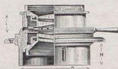
Helical Focussing Mount H
