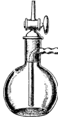
1104. — Chancel's Flask, for taking the specific gravity of gases. Each .. .. . 11/6
