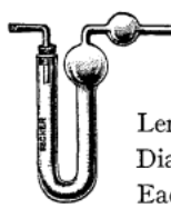
654.—Calcium Chloride Tubes, Marchand's form, with cork and leading tube.
