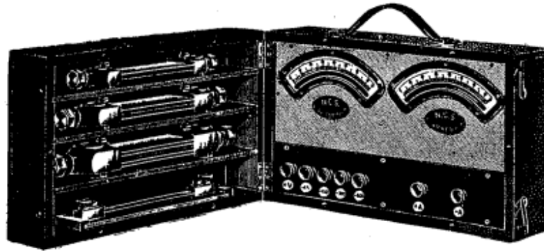
Combined Ammeter and Voltmeter, moving coil Type. FIG. 5.
