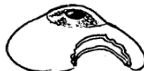
Reform or Full Back Eye. Broken to show Double Wall.
