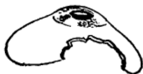
Shell Eye Broken to show Single Wall Construction.
