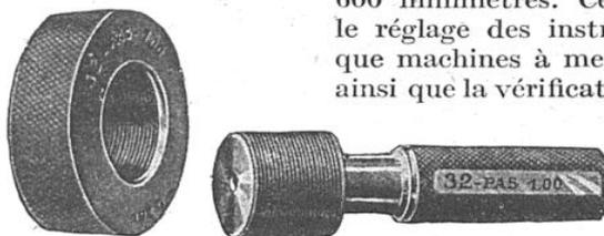
CALIBRE DE FILETAGE POUR ROBINETTERIE DE 32 MILLIMÈTRES AU PAS DE 1.00
