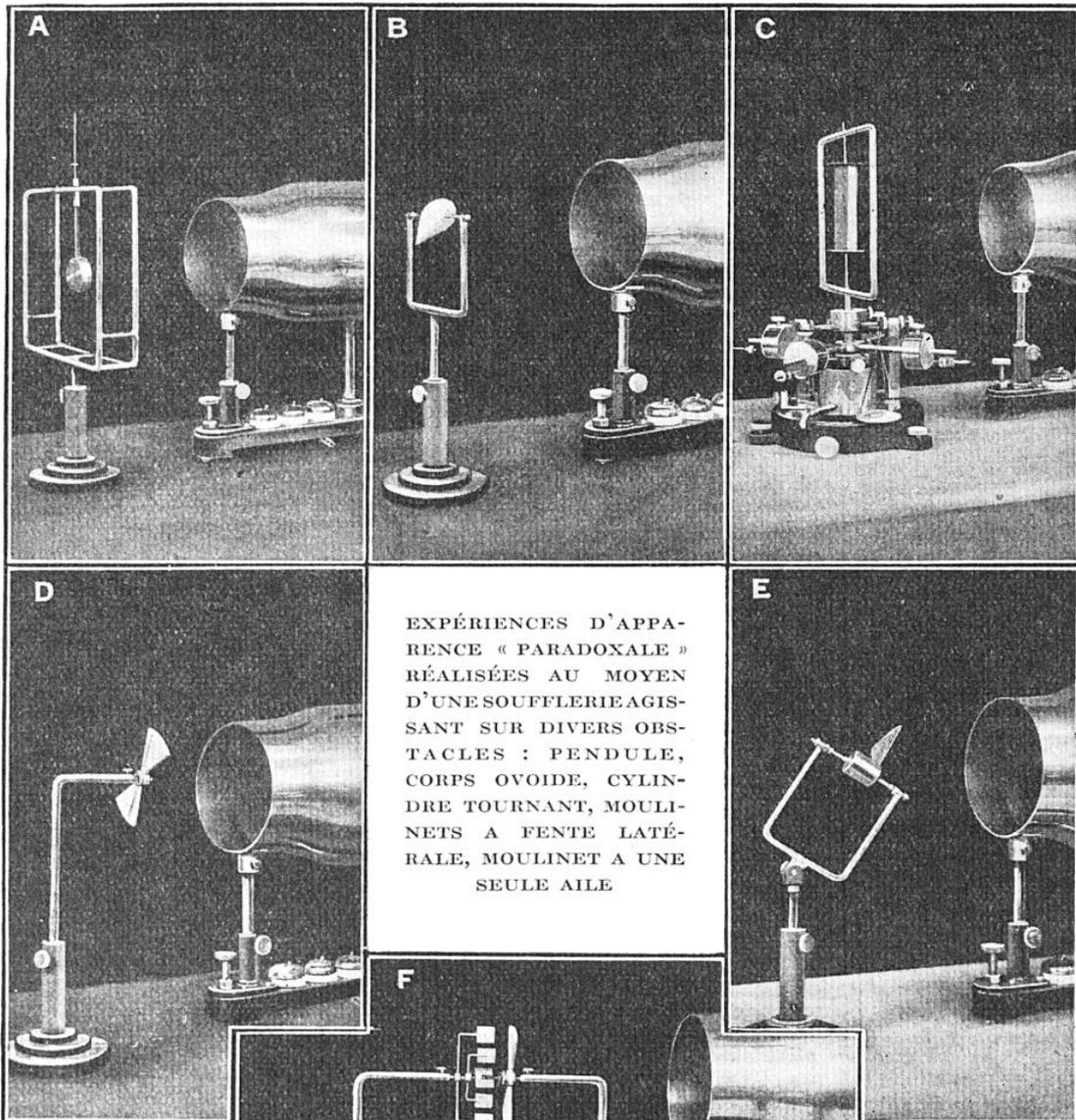
EXPÉRIENCES D'APPARENCE « PARADOXALE » RÉALISÉES AU MOYEN D'UNE SOUFFLERIE AGISSANT SUR DIVERS OBSTACLES : PENDULE, CORPS OVOÏDE, CYLINDRE TOURNANT, MOULINETS A FENTE LATÉRALE, MOULINET A UNE SEULE AILE
