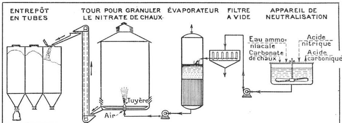
FIG. 10. — SCHÉMA D'ENSEMBLE DE LA FABRICATION DU NITRATE DE CHAUX
