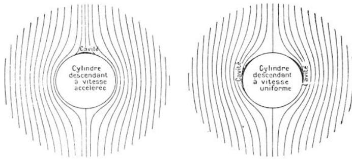
FIG. 8. — COMMENT APPARAISSENT LES CAVITÉS AUTOUR D'UN OBSTACLE SE DÉPLAÇANT DANS UN FLUIDE
