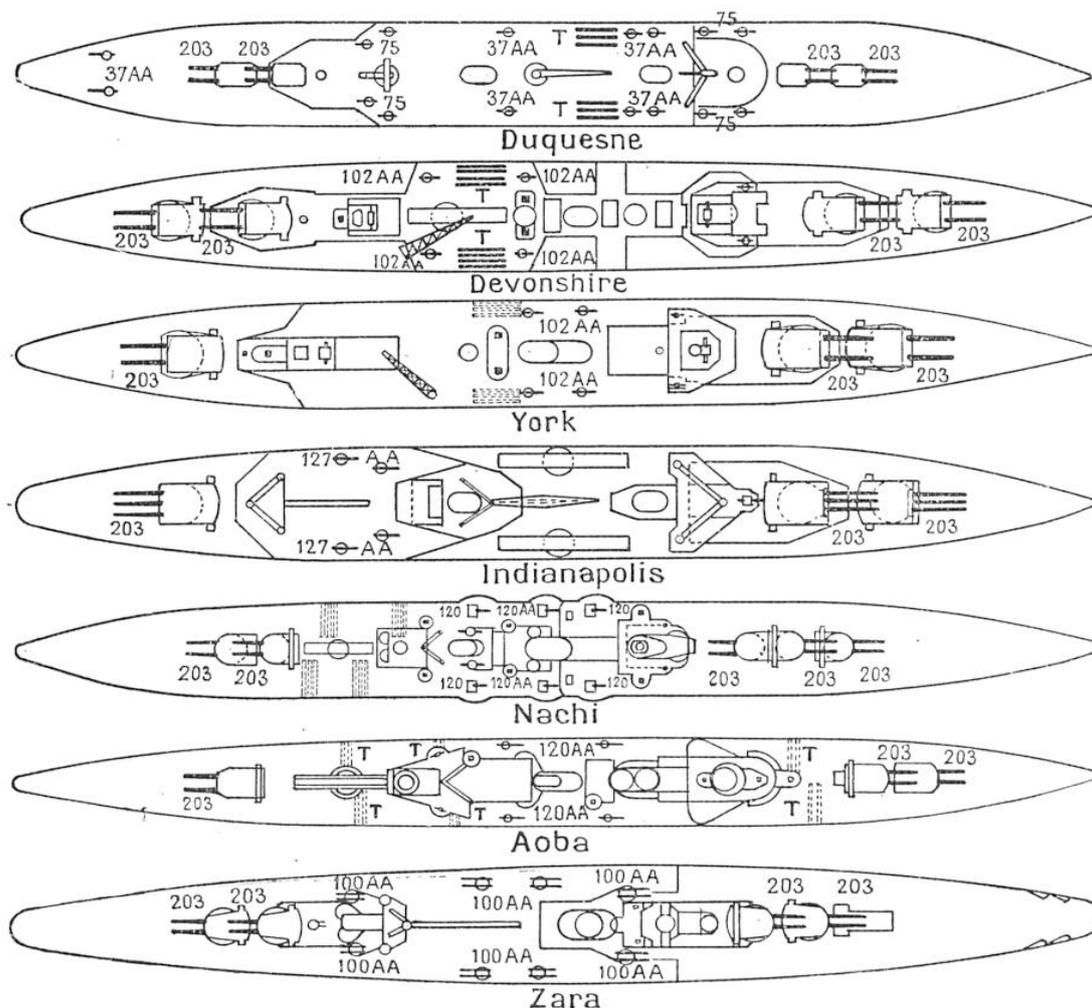
FIG. 4. — SCHÉMA MONTRANT LES CARACTÉRISTIQUES DES PRINCIPAUX BATIMENTS INDICUÉS SUR LE TABLEAU PRÉCÉDENT ET RENTRANT DANS LA CATÉGORIE DES CROISEURS DE 1<sup>re</sup> CLASSE
