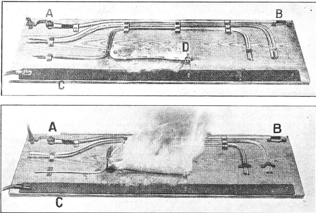
FIG. 1 ET 2. — EXPÉRIENCE DE M. OTTO MONTRANT COMMENT UN DÉFAUT D'ISOLEMENT D'UN CABLE PEUT PROVOQUER UN COMMENCEMENT D'INCENDIE SUR UN FIL ÉLOIGNÉ DU CABLE
