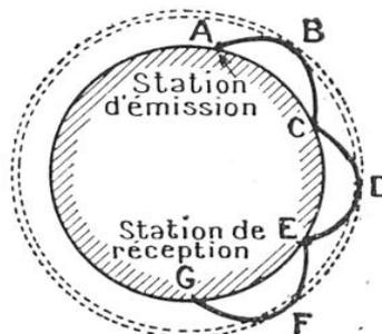
FIG. 2. — ABCDEFG : TRAJET D'UN FAISCEAU DE RAYONS DE FORCE ÉLECTRIQUE, AVEC RÉFLEXIONS SUCCESSIVES DANS L'ATMOSPHERE ET SUR LE SOL
