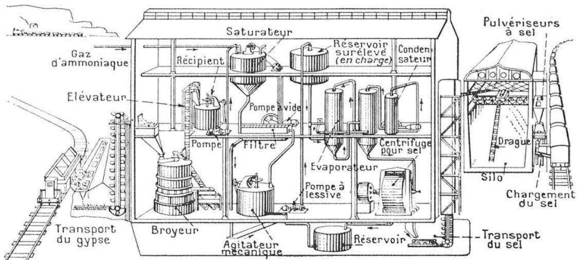
FIG. 5. — FABRICATION DU SULFATE D'AMMONIAQUE, D'APRÈS LE PROCÉDÉ HABER-BOSCH
