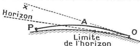
FIG. 3. — P A O : TRAJET D'UN FAISCEAU COURBÉ PAR LE MIRAGE ET QUI FAIT VOIR, A UN OBSERVATEUR EN O, LA LANterne D'UN PHARE P SITUÉ AU DELA DE LA LIMITE DE L'HORIZON. OX, DIRECTION DANS LAQUELLE EST VUE DE O LE PHARE P
