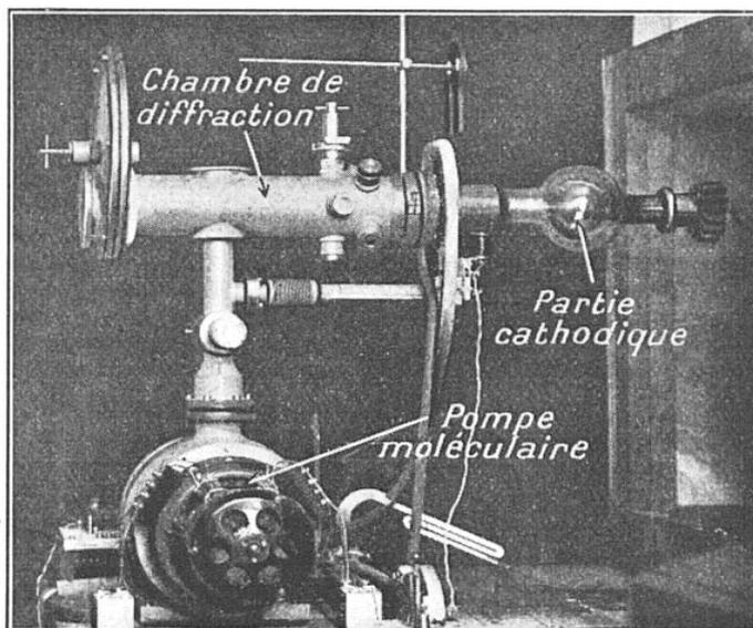
FIG. 6. — RÉALISATION D'UN APPAREIL POUR LA DIFFRACTION D'ÉLECTRONS RAPIDES (J.-J. TRILLAT)
