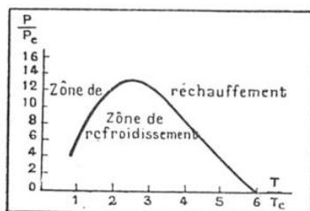
FIG. 2. — CETTE COURBE DÉFINIT LES CONDITIONS DANS LESQUELLES UN GAZ DOIT SE TROUVER POUR QUE SA DÉTENTE ENTRAÎNE SON REFROIDISSEMENT
