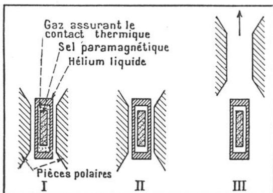
FIG. 5. — COMMENT ON S'APPROCHE AU VOISINAGE DU ZÉRO ABSOLU PAR DÉSAIMANTATION D'UN CORPS PARAMAGNÉTIQUE
