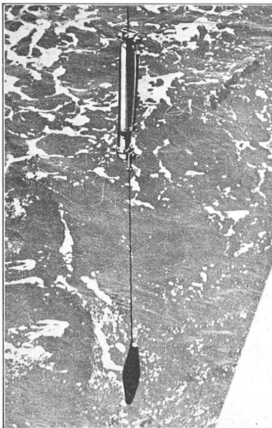
FIG. 6. — LA BOUTEILLE HANSEN SERVANT A LA PRISE D'EAU MARINE AUX FINS D'ANALYSE
