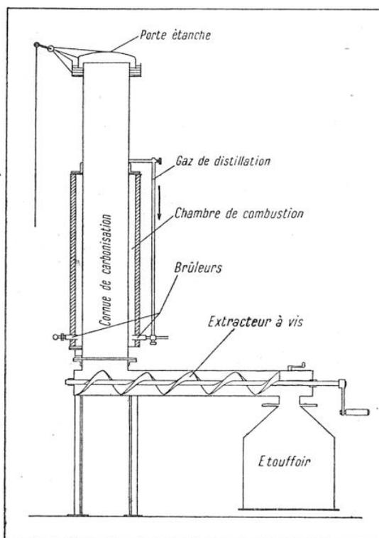
FIG. 6. — SCHÉMA DE PRINCIPE D'UNE CORNUE DE CARBONISATION CONTINUE
