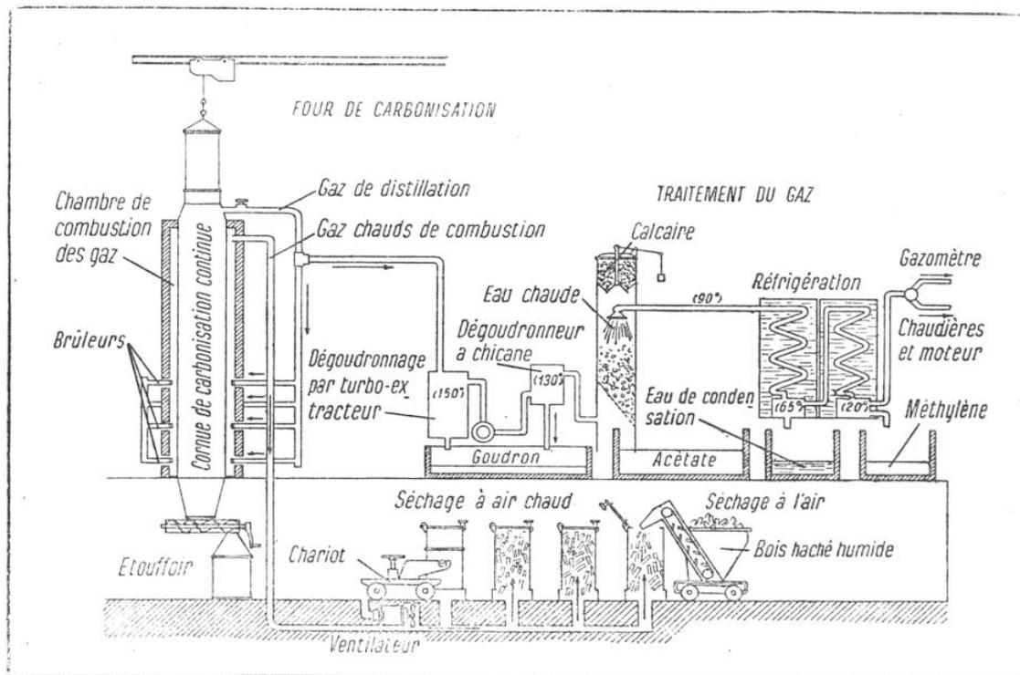
FIG. 9. — SCHÉMA DE PRINCIPE D'UNE USINE DE PRODUCTION DE CARBURANTS SOLIDES ET LIQUIDES
