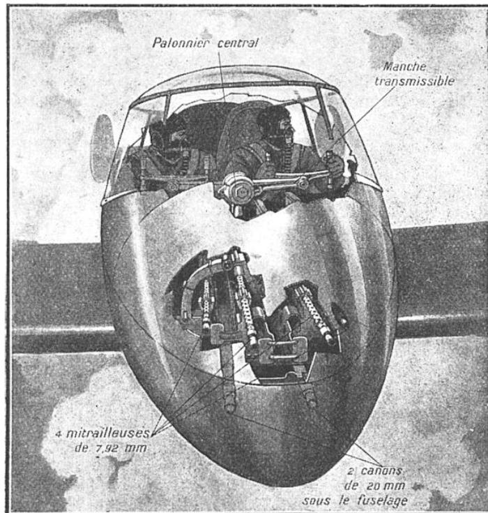
FIG. 6. — L'ARMEMENT DU MESSERSCHMITT 110
