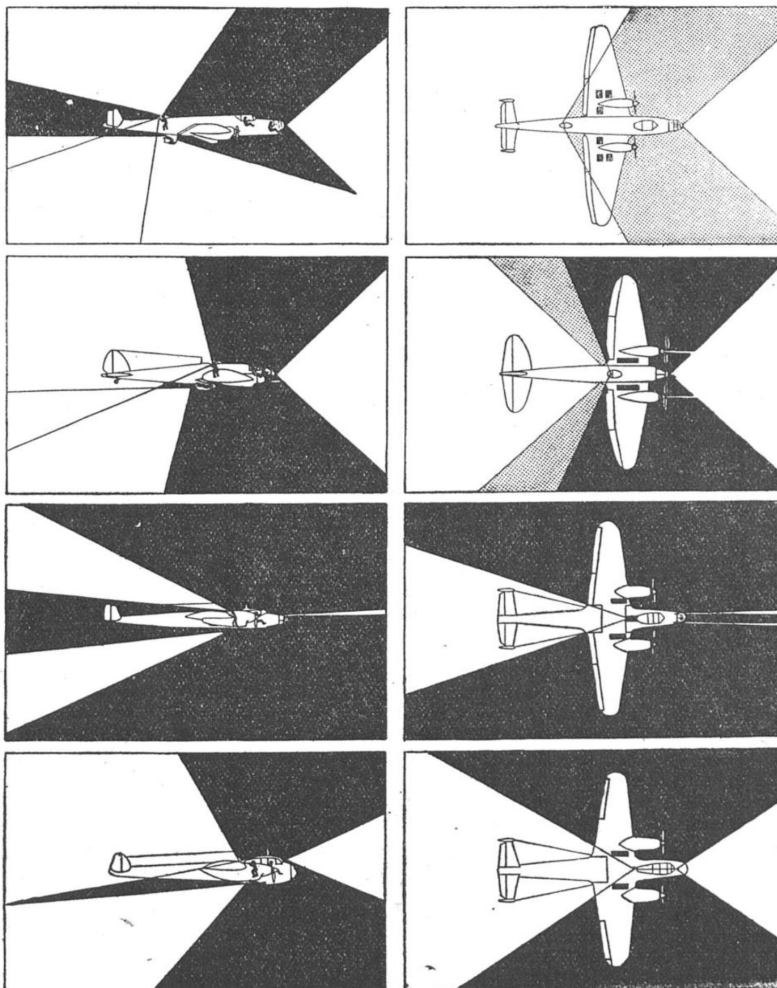
FIG. 4. — CHAMPS DE TIR ET ANGLES MORTS DE DIFFÉRENTS APPAREILS ALLEMANDS DE BOMBARDEMENT
