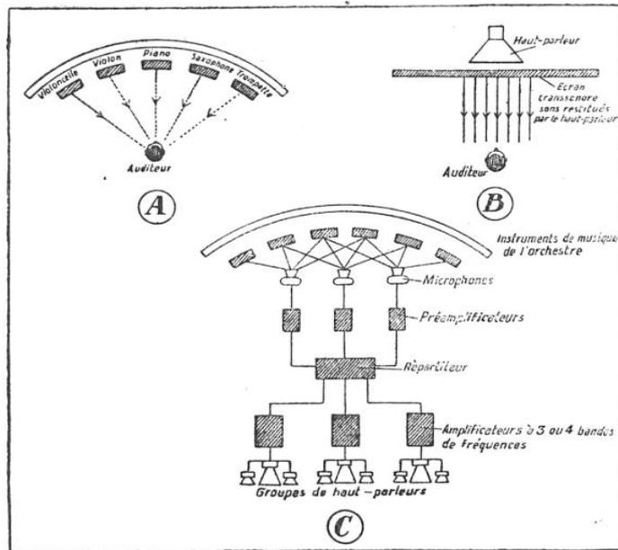
FIG. 11. — PRINCIPE ÉLÉMENTAIRE DE LA PRISE DE SON FRACTIONNÉE ET DE LA RÉPARTITION SONORE
