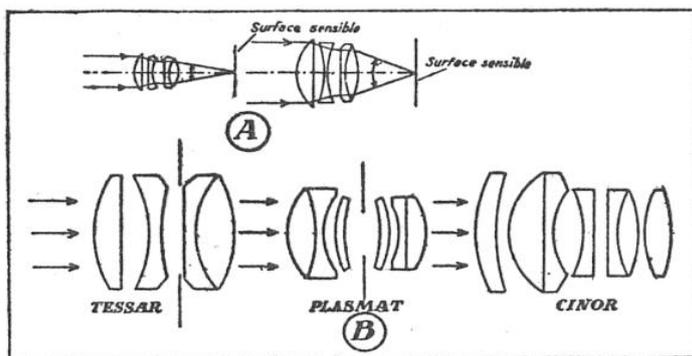
FIG. 1. — LA LUMINOSITÉ DES APPAREILS DE CINÉMA
