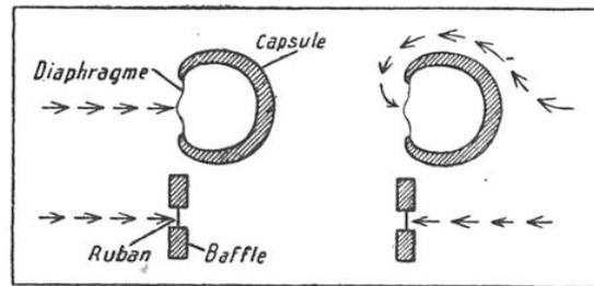
FIG. 6. — PRINCIPE DU MICROPHONE CARDOÏDE
