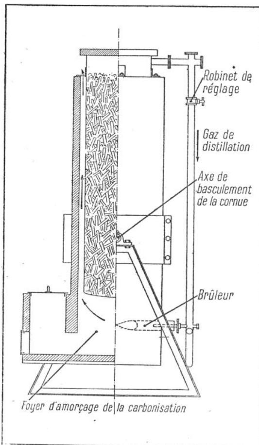
FIG. 2. — FOUR BASCULANT DE CARBONISATION DU BOIS EN VASE CLOS
