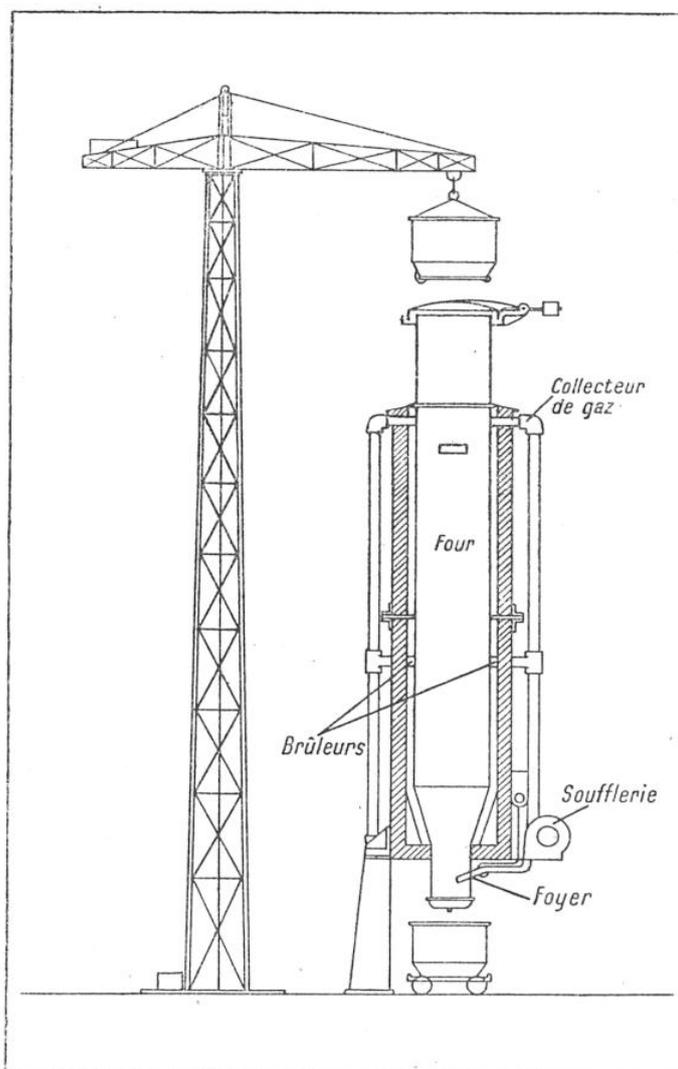
FIG. 7. — INSTALLATION SEMITRANSPORTABLE DE CARBONISATION A FONCTIONNEMENT CONTINU
